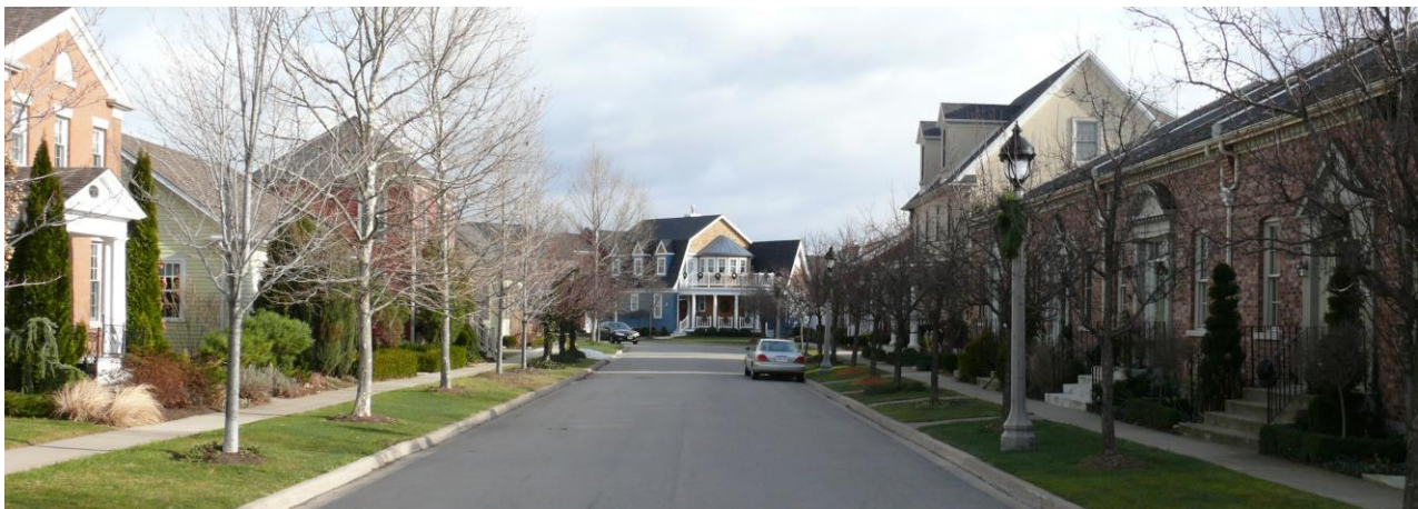
Figure 18: Well framed residential streetscape, Niagara-on-the-Lake, Ontario. Minimal front yard setbacks frame the street and create a comfortable pedestrian environment. A bend in the street creates a terminal vista furthering the sense of enclosure. This concept is described as an ‘outdoor room.’ Sidewalks, street trees and pedestrian scaled lighting also contribute to the pedestrian oriented character of the neighbourhood.
